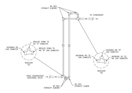
Figure 19: Double Riser Detail
